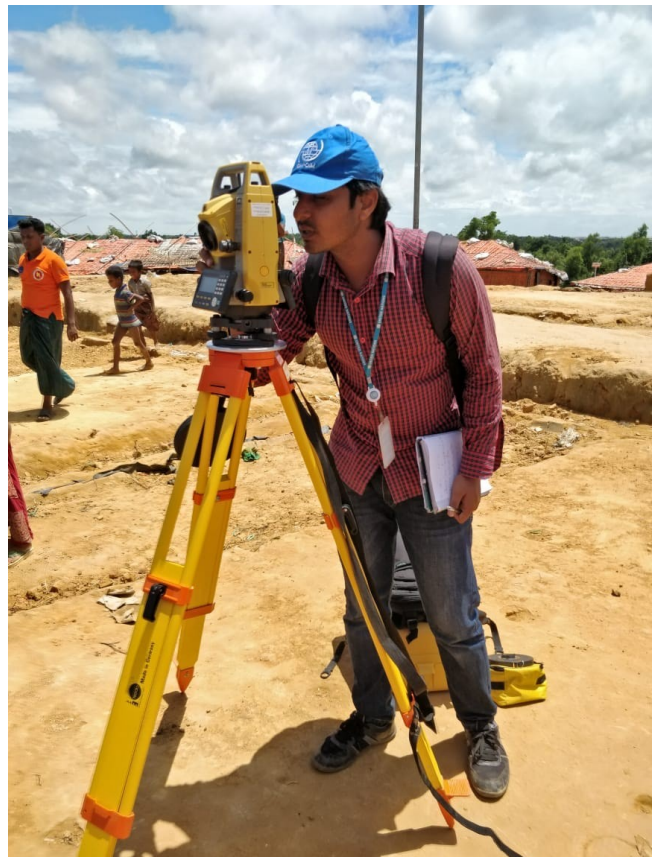
Topographic Survey in Camp 12 for the water supply system. ©IOM 2018
