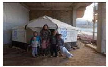
Note this version if the family tent is for cold climates / winter conditions. It is similar to the family tent apart from the fact that it has a steel frame. This frame makes it self standing, and hence more suitable for use on hard ground (or concrete).
